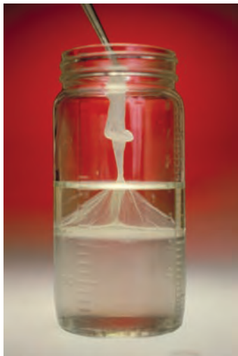
Figure 6.17 The rate at which the nylon is produced is controlled by limiting the surface area where the reactants in each layer can make contact.
